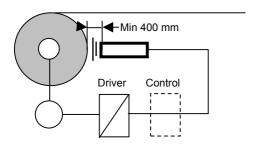
Reading roll diameter in the Web Tension Control application in order to exploit diameter information as torque reference or as PID compensation in closed loop solution with control. In this case setting should be:
